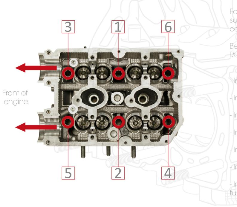
Follow the instructions below for torque settings and be sure to adhere to the diagram opposite, showing the correct tightening sequence.
